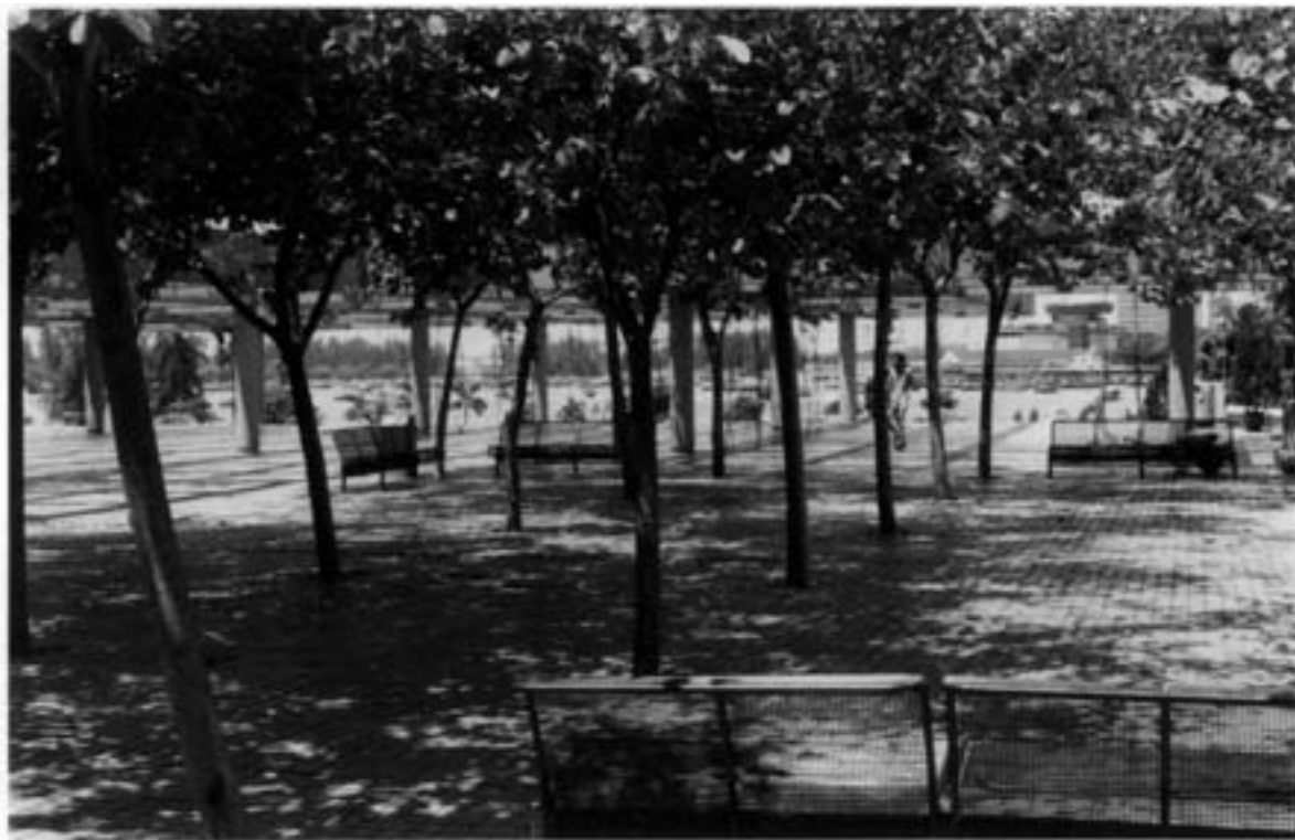
Bauhinia trees planted on a rooftop plaza in Singapore near a large shopping complex. Trees are recessed into the structure so that there are no raised planters.
